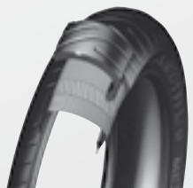
BELTED TYRE WITH RADIAL CARCASS (90 DEGREES)
