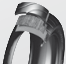
0°- STEEL BELTED TYRE WITH RADIAL CARCASS (90 DEGREES)
