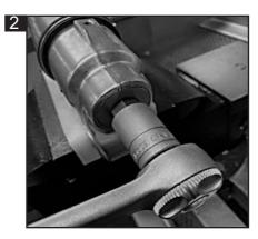
2: Uncrew the base valve assembly from fork foot using a 17mm hex. Oil remaining in the fork may leak out - have a suitable container to hand.
