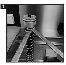
1: Remove the top cap from the piston rod assembly. Remove the main spring and empty fork oil into a suitable container.
