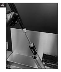
4: Remove the cartridge from the fork leg.
