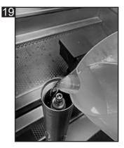
17: Install base valve assembly into fork foot. Apply green grease to o-ring.
