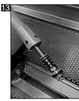
11: Select correct K-Tech piston assembly for fork leg, apply Loctite 2701 to thread and install into piston rod.
