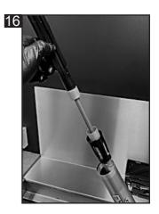
14: Install circlip onto piston rod.
