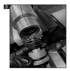
3: Remove the base valve assembly.
